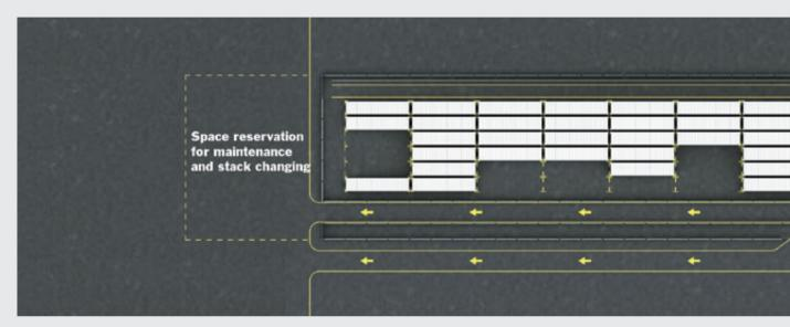
**THE BASIC ARTG CONTAINER STACK LAYOUT.** ARTG stack operations are side-fed. ARTG gantry movement is limited as much as possible. The truck drives to meet the ARTG for loading/unloading operations.
