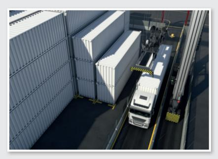
Truck loading and unloading is done by the remote operator in the Remote Operating Station (ROS). One remote operator can handle up to 6 ARTGs.
