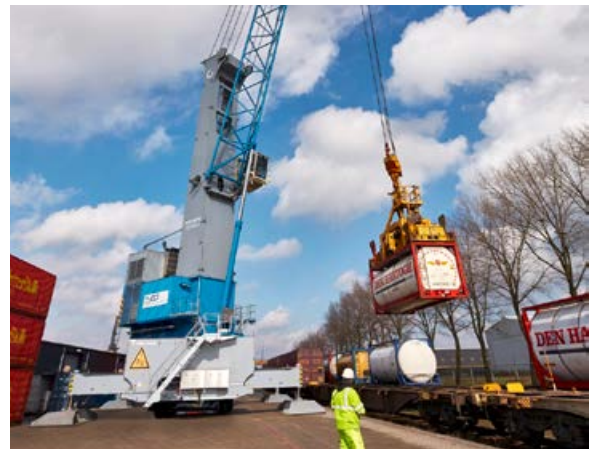
Utmost flexibility: Konecranes Gottwald Model 4 Mobile Harbor Crane unloading tank containers from freight cars and positioning them directly in the stack
