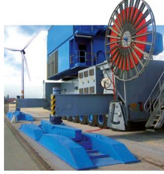
Since 1956, we have focused on the diesel-electric drive system generating power on board of the cranes. Thanks to this drive technology, external power from on-shore power grids can be used easily, forming an ideal match, since additional equipment for energy conversion is not required. This improves the eco-efficiency of our cranes further and allows surplus energy to be fed back into the grid.
