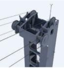
Ladders for safe ascent to the tower head. Extended platform for easy access to rope pulleys for maintenance work.
