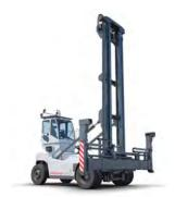
The purpose of the training is to provide the necessary knowledge to handle and operate the empty container handler (ECH) in order to handle and move empty containers in a safe and productive way.
