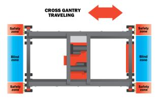
Figure 6 and 7. The safety zones are pre-programmed according to local regulations and your own yard requirements. Seen here: normal and cross gantry travel. "Rotate" is also available. In cross-gantry travel, the "blind zones" can be eliminated by adding more laser sensors.
