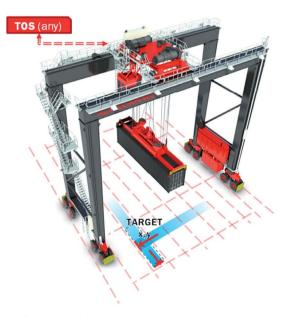
Figure 14. Auto-Positioning helps make load movements more precise.
