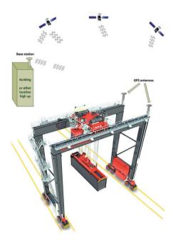
Figure 12. Auto-Steering creates virtual rails (the yellow lines) using on-board GPS receivers.
