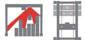
Figure 8. The Stack Profiling System remembers the layout of your container bay. Here is a sample layout from the side (left) and the top (right).
