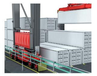
Figure 4. The busbar retrofit converts your RTG to fully electric operation. Power is supplied by a low, electrified fence.
