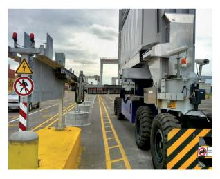
Figure 5. The Georgia Ports Authority (GPA) operates over 120 Konecranes RTGs including the fully electric busbar RTG pictured here at the Port of Savannah. The GPA plans to operate over 150 fully electric RTGs by 2022 via purchases of new electric RTGs and retrofitting existing RTGs.
