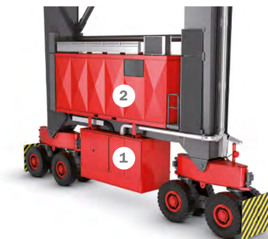
Figure 2. The diesel fuel saver is retrofitted in the genset enclosure (1) while the necessary modifications to the electrical systems are made in the e-house (2) above it. Some software modifications are also done at the same time.
