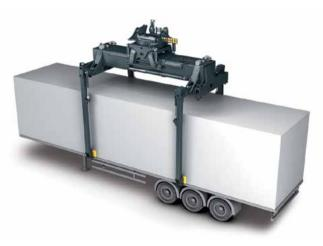
**ELME 857-HPS in action** Legs shown in unfolded position with a trailer being lifted.
