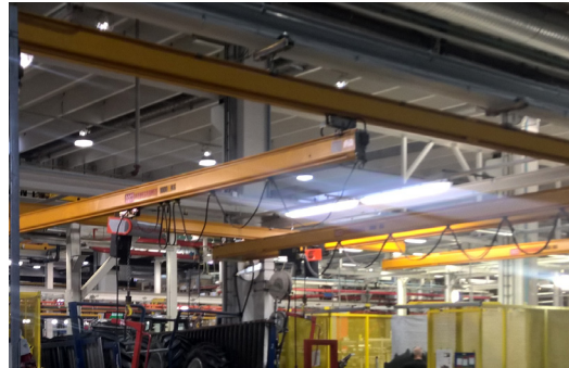
Konecranes XM steel workstation cranes equipped with a CLX electric chain hoist.
